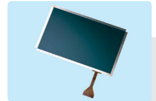
Automotive capacitive touch panel
